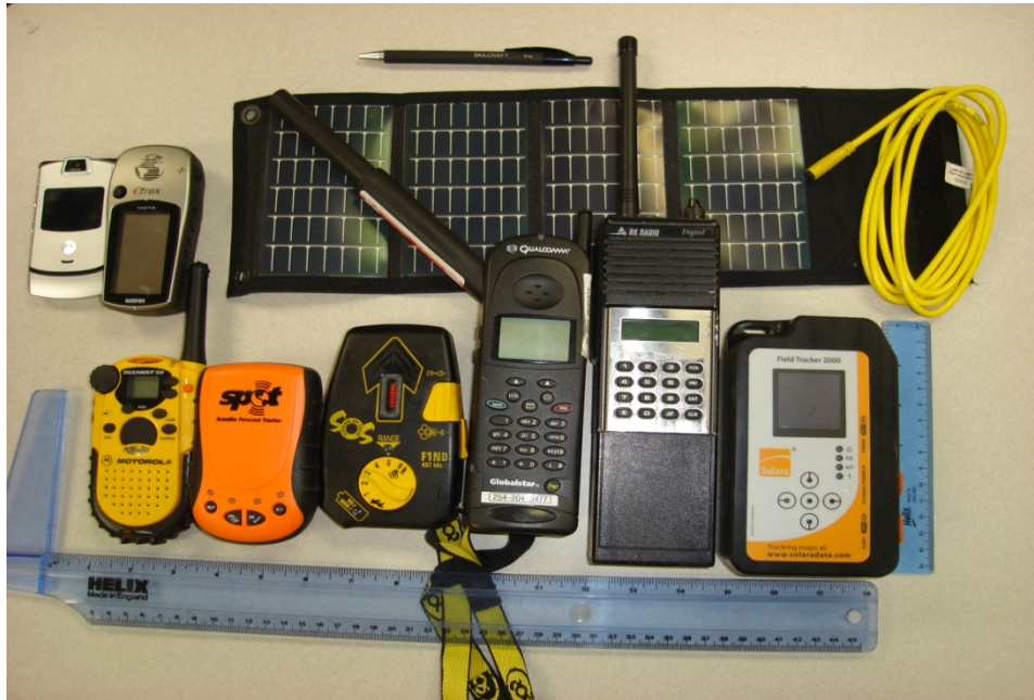
Photo showing from left to right: Cell Phone, Garmin E-trex GPS, Solar panel for SOLARA, Motorola Talkabout, SPOT, SOS Avalanche Transceiver, Qualcomm Satellite Phone, BK Radio, SOLARA.
