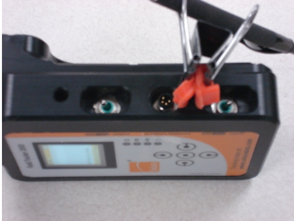
SOLARA showing recessed-covered toggle switch & charging connection.
