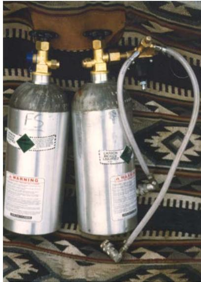
While transporting in a vehicle you must allow for adequate ventilation. In the back of an open pickup properly secured is best. If you must transport in an enclosed vehicle, windows must be opened for ventilation in the event of a product leak. While CO<sub>2</sub> is very safe in regards to flammability, it does pose an asphyxiation threat in an enclosed environment. Maintain adequate ventilation where you store the CO<sub>2</sub> cylinders when not in use.
