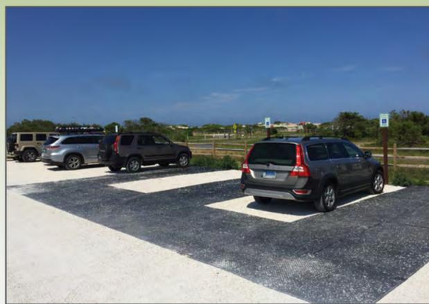
In response to accelerated shoreline erosion and greater storm impacts, Assateague Island National Seashore adopted climate-conscious solutions for beach facilities, including parking areas constructed from native clay and clamshell that can be reused in post-storm repairs. NPS Photo
