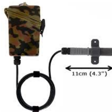
Figure 2. TRAFx Infrared Trail Counter .
