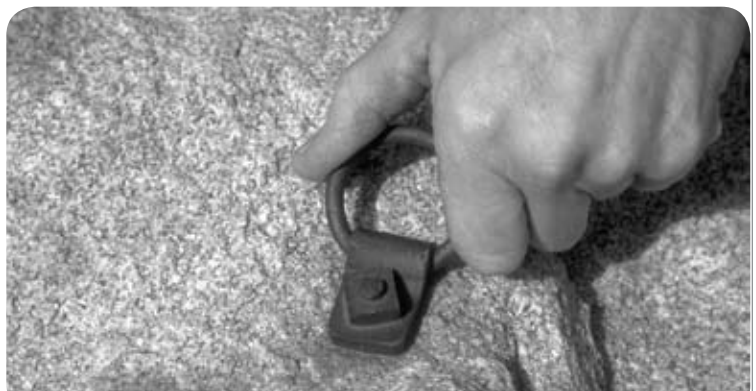
Photo of a weathered fixed safety anchor over 30 years old. Old anchors can be removed cleanly and the same hole used to place a new anchor of a higher standard of safety. If use of the anchor is redundant the hole can be filled with a resin and natural rock dust mixture so as to be indiscernible. Photo: © Access Fund Collection
